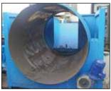
The Baughans Refiner Barrel unique design with neoprene screens with a cleaning flipper enabling screening of Compost, soils aggrigates etc.
