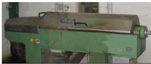
Photo 11: Decanter centrifuge and separated liquid and fibre
