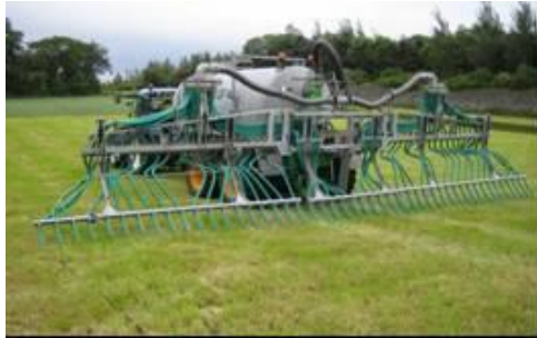
Photo 9: Trailing hose application places slurry on the surface
