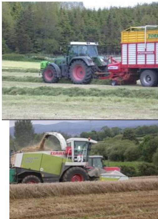
Photo 2: Grass harvesting with a self-loading forage wagon and whole crop wheat harvesting with a self-propelled forage harvester
