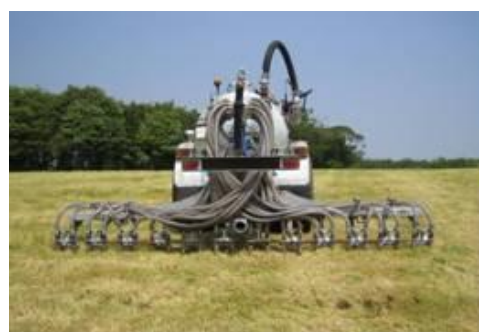
Photo 8: Trailing-shoe application places digestate on the soil surface beneath any foliage
