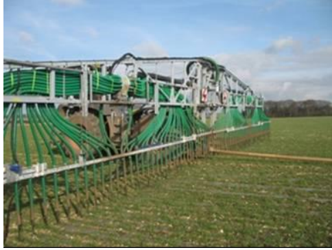
Photo 3: Trailing hose application of digestate to cereal
