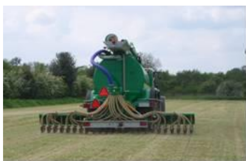
Photo 7: Shallow injector places digestate just below the soil surface
