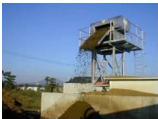
Photo 10: Rotary screen separator (copyright required www.lintonsolutions.com )
