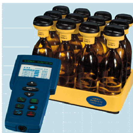
Figure 14. Oxitop system for pressure monitoring.
