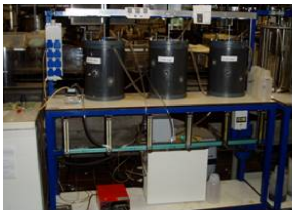
Figures 7a and b. CSTR reactors: experimental set-up and schematic representation
