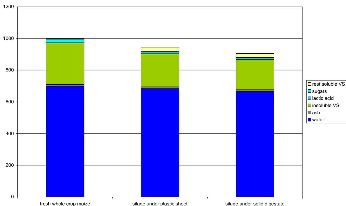
**Figure 2:** Changes in composition of whole crop maize after ensiling under coverage with plastic sheet or digestate, respectively. The values are based on 1 000 kg of fresh material and include the losses during the ensiling process.
