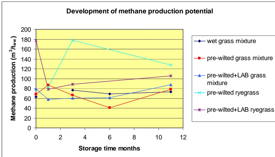
Figure 7: Change of methane production potential (m<sup>3</sup>/t<sub>ww</sub>) during storage of grass and ryegrass in bales. Mass loss during pre-wilting was taken into account.
