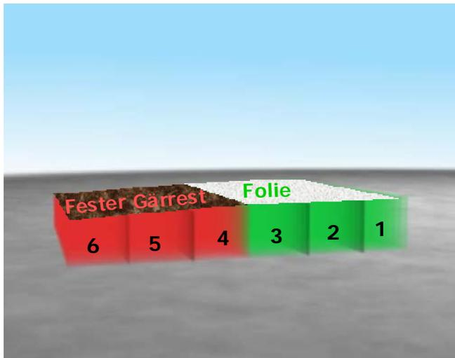
**Figure 1:** Division of the silo into sections. The sections covered with plastic sheet are marked in green, while the sections covered with solid digestate are marked red.
