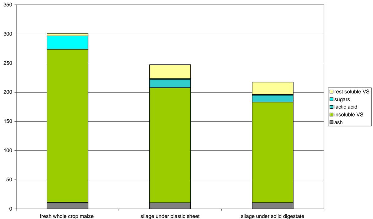
**Figure 3:** Changes in composition of the solids fraction in detail. The values are based on 1 000 kg of fresh material and include the losses during the ensiling process.
